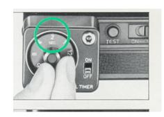
·By resetting the ON/OFF switch of the Contax Interval Timer to "OFF", you can immediately resume normal film-winder-assisted photography.
