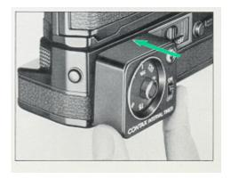
The Contax Interval Timer is used by plugging into the sockets of the Yashica Winder. Before shooting the series of photos with the aid of the Contax Interval Timer, take a couple of blank shots to determine whether the interval timer and film winder systems function properly. If the test lamp of the film winder comes on each time after the film is advanced, it means that the systems are functioning properly.
